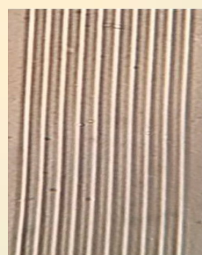
Diffraction grating on the MC layer recorded by a digital camera through the optical microscope
