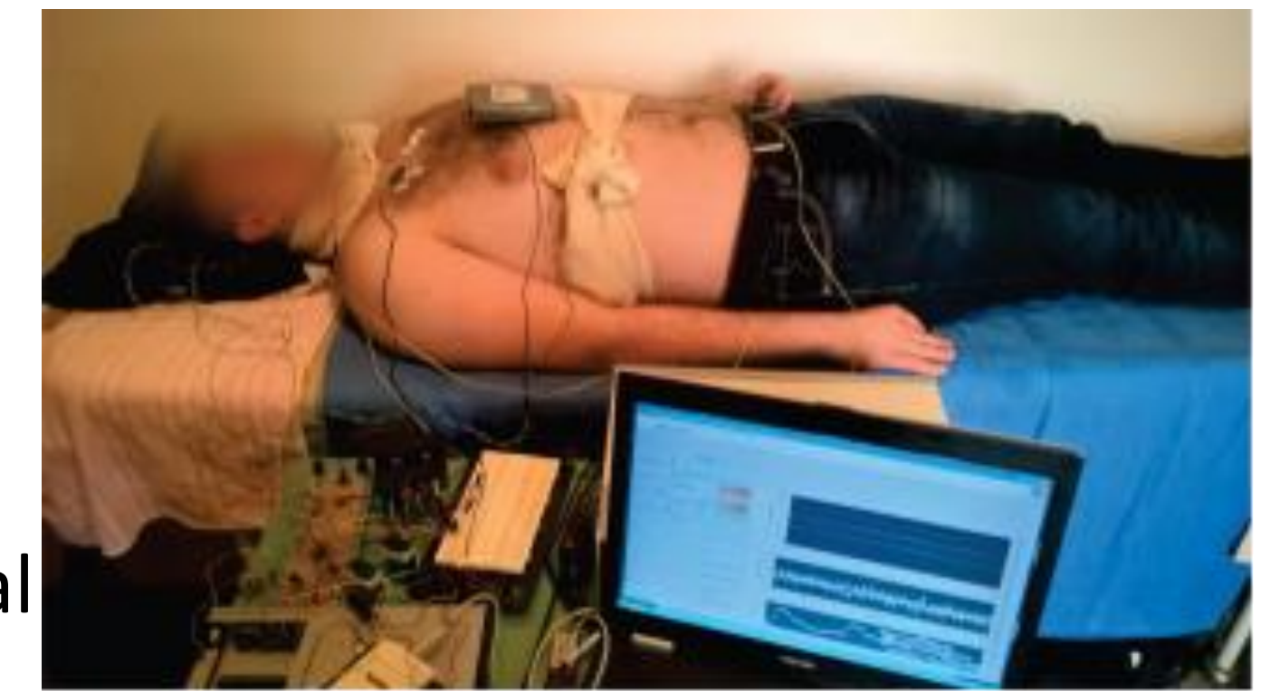
Fig. 6. Healthy subject in measuring supine position with LPG, ECG and PCG sensor
