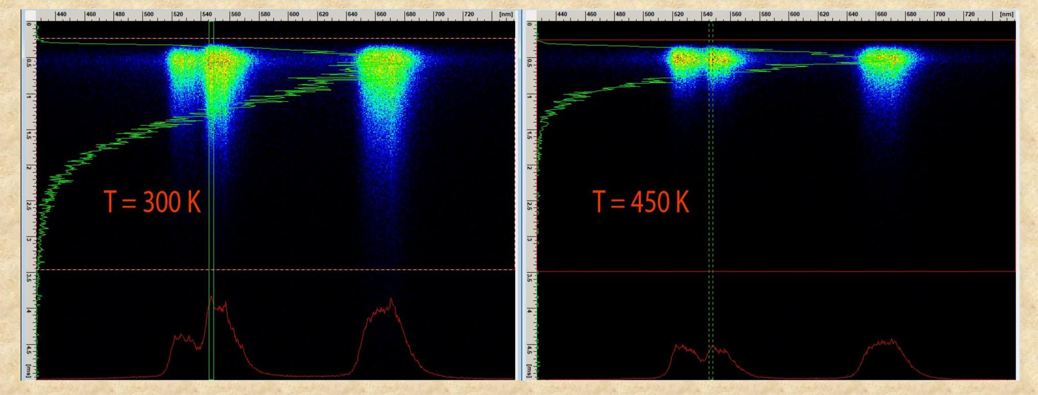
Streak images of Gd<sub>2</sub>O<sub>3</sub>:Er<sup>3+</sup>,Yb<sup>3+</sup> excited at 980 nm, at different temperatures. Images are presented in pseudocolor where different colors correspond to different intensities. Vertical axis corresponds to time, here it is 5 ms from the start to the end of streak image. Horizontal axis corresponds to wavelengths of optical emisssion.
